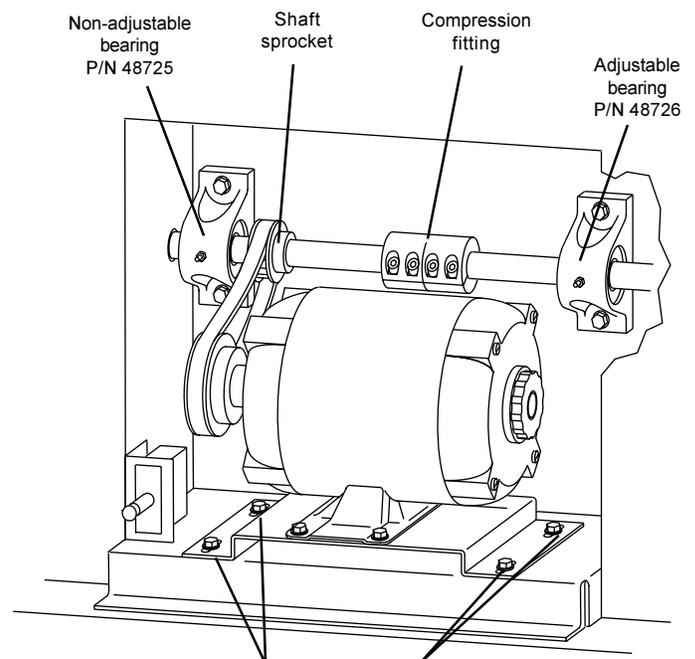
Loosen four (4) screws to adjust motor position and belt tension
